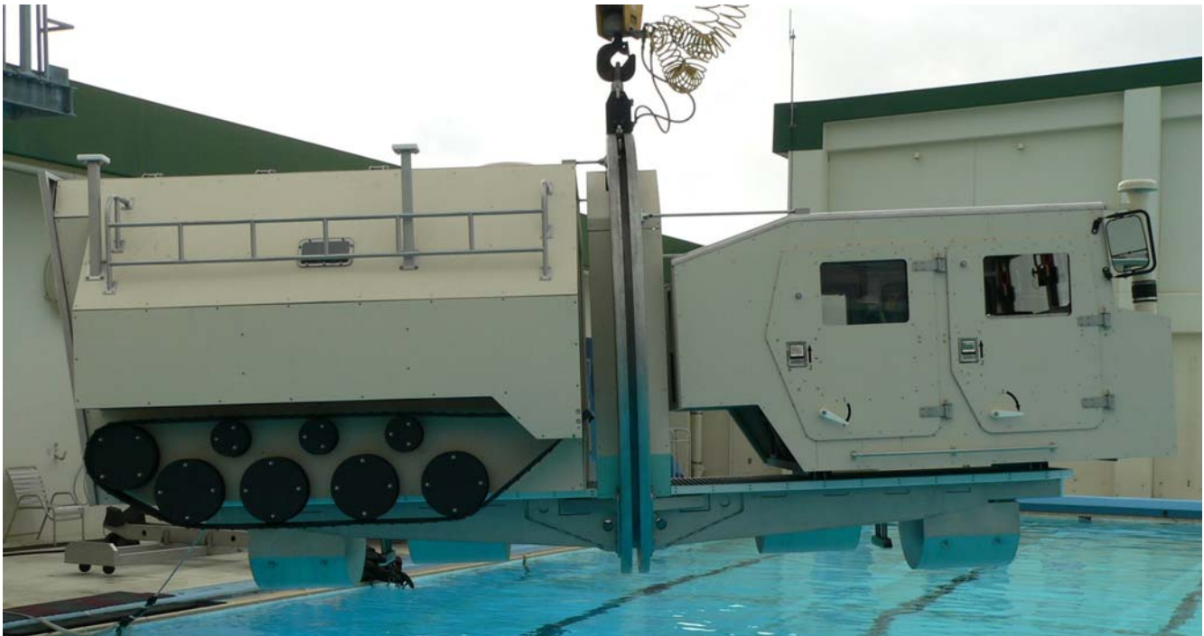
Multi-Platform METS™ (MPM™) with High Mobility Multi-purpose Wheeled Vehicle (HMMWV) and Amphibious Assault Vehicle (AAV) Modules
