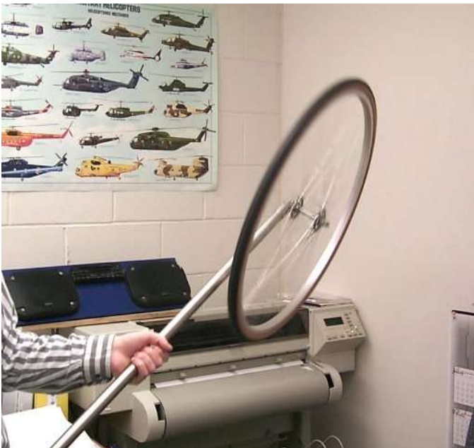
Device Used to Demonstrate the Gyroscopic Effect of the Sea State
