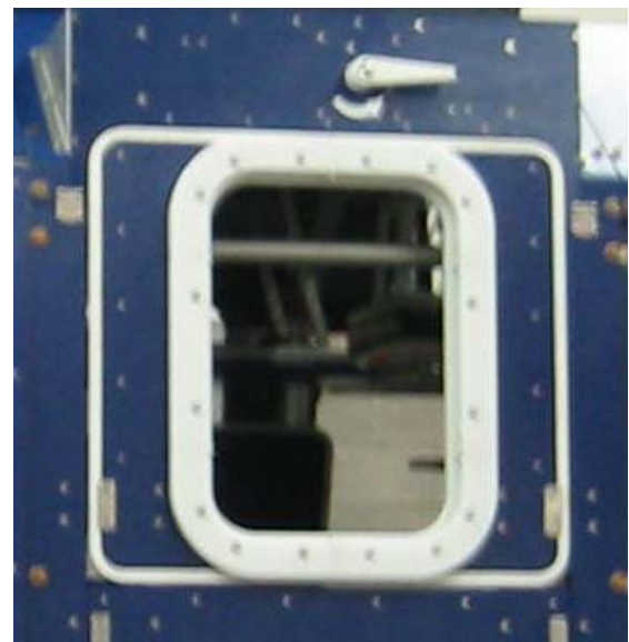
H-53 Cabin Mechanical Door with H-53 Push-Out Window
