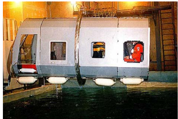
1987 to 1988 Survival Systems Develops the First Modular Egress Training Simulator (METS™) Prototype
