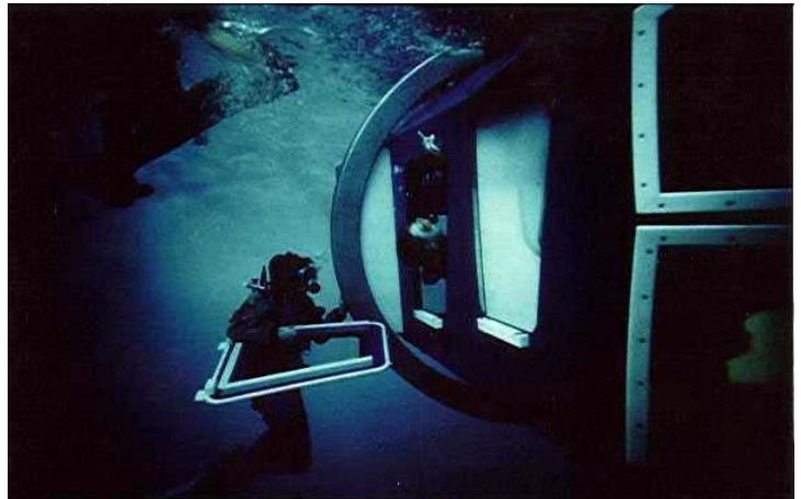
Jettisoning Emergency Escape Exits from the METS™
