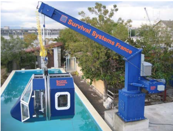
4000 Lb Single-Drive Jib Launch, Operation, and Recovery Systems (LORS)
