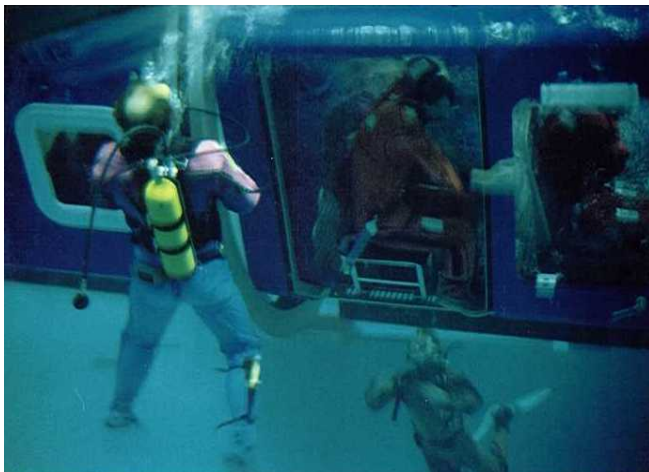
Jettisoning Emergency Escape Exits from the METS™
