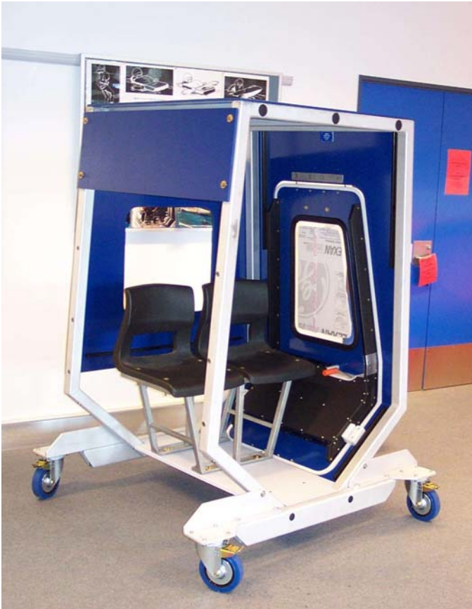
Classroom Egress Trainer Used to Demonstrate Egressing
