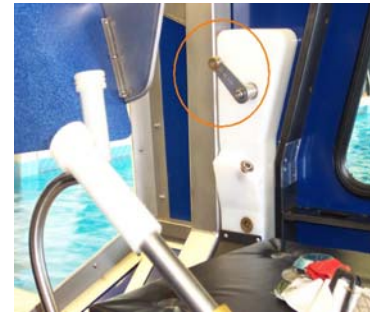
Exit Release Mechanism for BO-105
